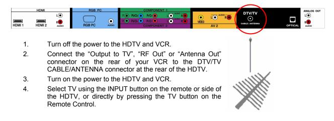
Note: If you have an off-air antenna or cable TV, connect it to the "Antenna In" connector on the rear of your VCR.
